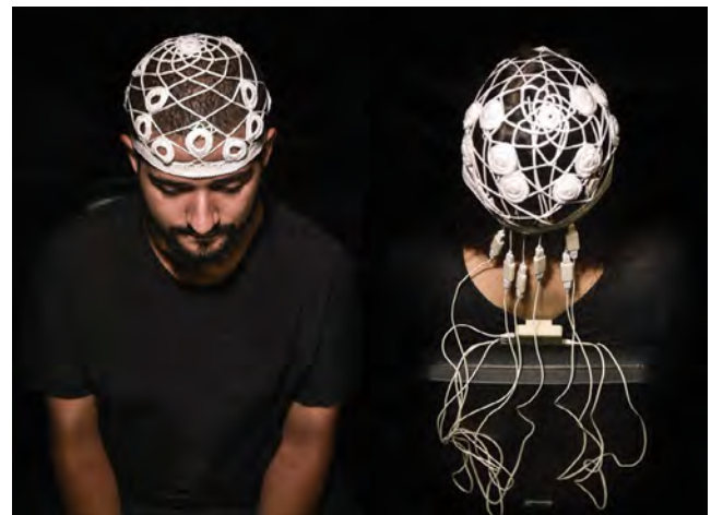
Figure 3. The Schizocap photos show the front and top electrode positions based on the 10-20 System, worn by a man and woman, respectively. The right photo shows the final version of the prototype. Photo by Thiago Barcelos
