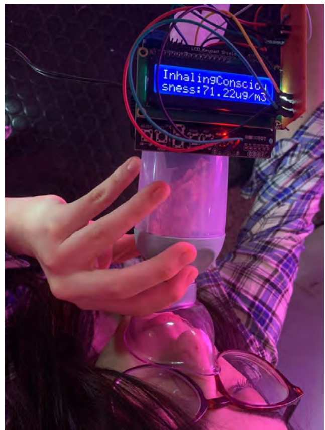
Figure 10: Installation components for the ISEA 2020 online version: Pocket Inhaler's vapor chamber (Mini Handheld nebulizer), having a sample of the Terminalia catappa 's bark inside together with a particles sensor system (Arduino, sharp dust sensor, LCD 16x2) that allows the audience to visualize the amount of particles being inhaled.(photo by the artist)
