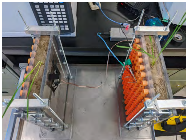
Figure 4. Rhizotrons with electrical signal amplifier (developed with Martin Peach). Sampling sounds through septa using electrodes. © photo Sandra Volny.
