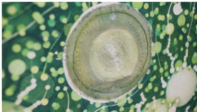
Figure 7. Speakers made with silver wire and neodymium magnets hand-stitched onto cotton canvas. Courtesy of artists.
