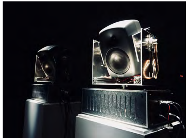
Figure 1. speaker.motion_2 An extended loudspeaker system capable of real-time pan and tilt movement. Image provided by the artist.
