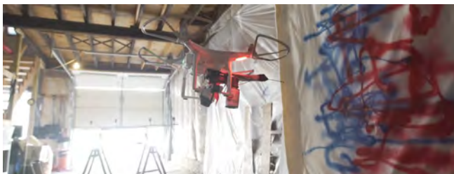
Figure 1. Human-drone painting setup. Real-time movements of the artist are captured and merged with the drone's native movement patterns to create final strokes.
