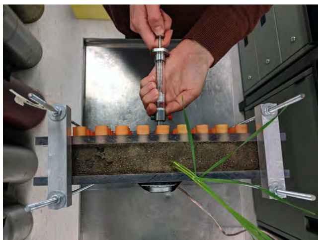
Figure 2. Rhizotrons exposed to underwater sounds through transducer. Sampling gas through septa using a syringe. © photo Sandra Volny.
