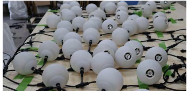
Figure 2. (a) One of the individual boards used in the Murmuration artwork and (b) a set of complete units ready for testing in the workshop; each unit incorporates board, speaker, housing and power socket.
